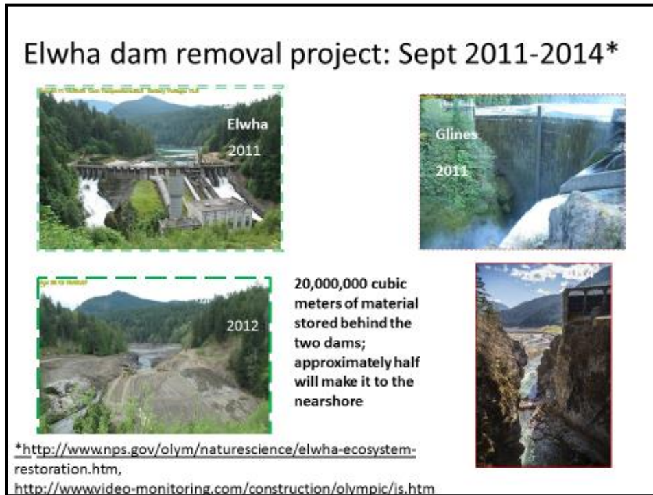
Figure 1: Photos showing the progress of the Elwha dam removal, which began in September of 2011 and ended in the summer of 2014.
